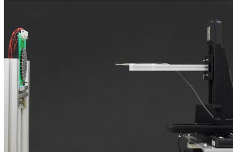
**Fig. 4.** Experimental setup for the measurement of the sound pressure. A microphone was attached to the 3D stage.
