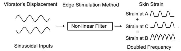
Fig. 10 Schematic of the ES non-linear filter.
