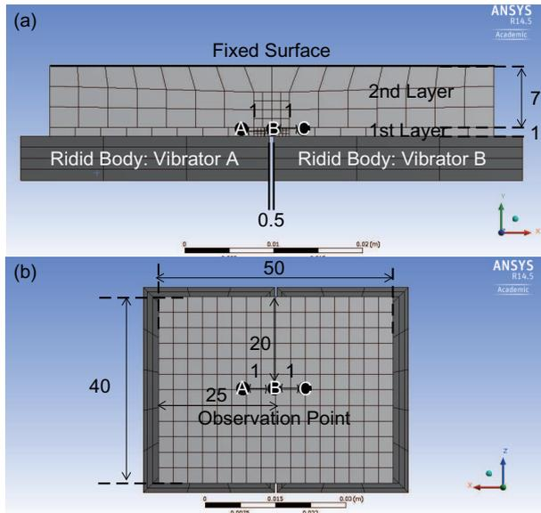
Fig. 6 Finite element skin model. (a). Front view. (b) Top view.
