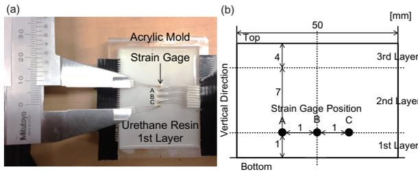
Fig. 2 Skin sensor. (a). Horizontal location of strain gages. (b). Cross section sketch of the skin sensor.
