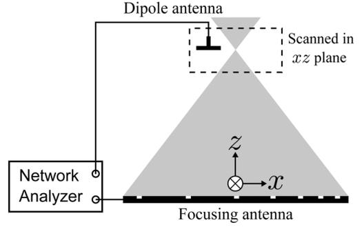
Fig. 4. Experimental setup. A dipole antenna is moved in  $xz$ -plane at 2-mm intervals to map the power density distribution.
