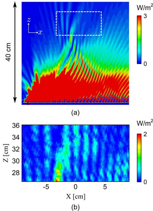
Fig. 7. Power density distribution maps at 18 GHz. (a) Simulation and (b) measurement. The measured area in which the color bar is valid is the same as Fig. 5.
