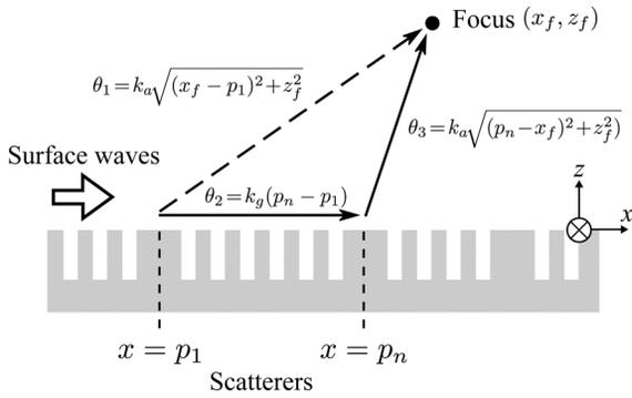
Fig. 3. Principle of focusing based on waveguide scattering. If the phase difference between the solid line and the dotted line equals to a multiple of  $2\pi$ , the waves interfere constructively, and a focus is generated.
