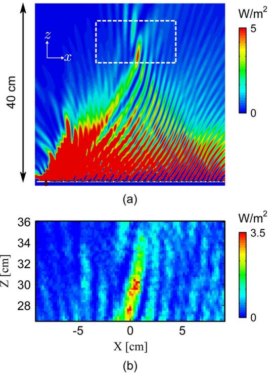
Fig. 5. Power density distribution maps at 20 GHz. (a) Simulation and (b) measurement. The measured area ( $-9$  cm  $\leq x \leq 9$  cm,  $y = 0$  cm,  $26.6$  cm  $\leq z \leq 36$  cm) in which the color bar is valid is indicated by the dashed square in upper figure.
