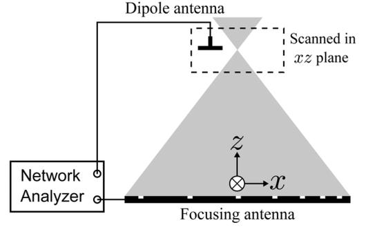
Fig. 4. Experimental setup. A dipole antenna is moved in  $xz$ -plane at 2-mm intervals to map the power density distribution.
