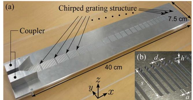
Fig. 1. Photograph of the fabricated focusing antenna. (a) Overview of the device and (b) enlarged view of the surface. The hole dimensions are as follows:  $s = 15$  mm,  $a = 1.35$  mm,  $h = 1.2$  mm, and  $d = 2.7$  mm.
