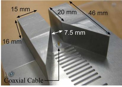
Fig. 2. Coupler to excite the waveguide from a coaxial cable. Metallic walls suppress unwanted backward radiation. An inner conductor of the coaxial cable lengthened by 2.4 mm is inserted from the backside of the aluminum plate.
