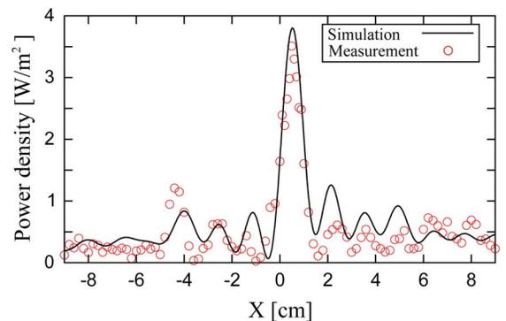
Fig. 6. Profile of the focus at 20 GHz at  $z_f = 30$  cm. The full width at half-maximum of the focus is about 9.7 mm, which equals to  $0.65\lambda$ .
