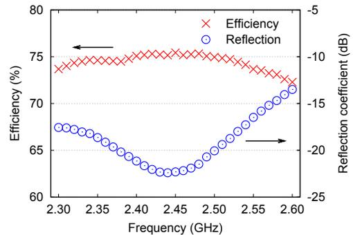
Fig. 7. Measured conversion efficiency and reflection coefficient versus frequency. The input RF power was fixed at 20 dBm. The peak efficiency is 75.4% at 2.45 GHz.
