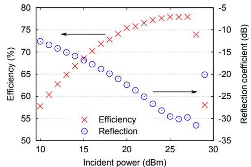
Fig. 8. Measured conversion efficiency and reflection coefficient versus input power. The RF frequency was fixed at 2.45 GHz. The peak efficiency is 77.9% at 27 dBm. Above 28 dBm, the output voltage (not shown here) saturates and the efficiency drops steeply, due to the breakdown voltage of the diodes.
