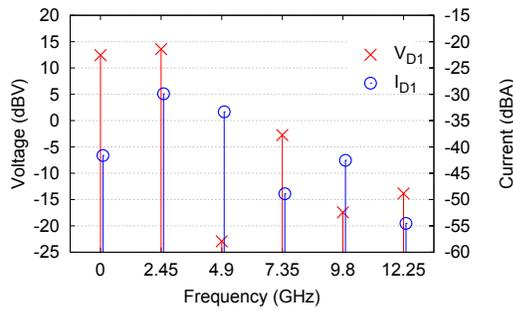
Fig. 4. Spectra of the simulated voltage and current across the diode  $D_1$ . The reference values are 0 dBV = 1 V and 0 dBA = 1 A.
