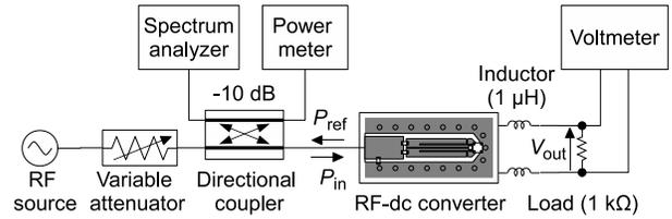
Fig. 6. Schematic illustration of the measurement setup. The frequency and the power of the microwave fed into the circuit are swept and the corresponding dc output are measured.
