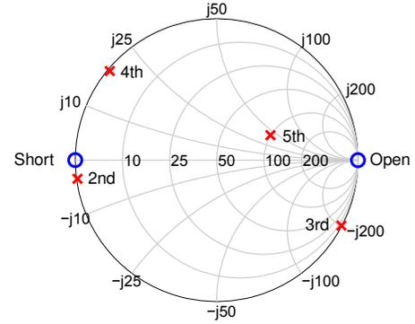
Fig. 3. Harmonic terminations of each diode. The terminations at the second and the fourth harmonics are approximately short, and one at the third harmonic is approximately open. The reflection coefficient at the fifth harmonic frequency is relatively low, because no filter is designed for this frequency.
