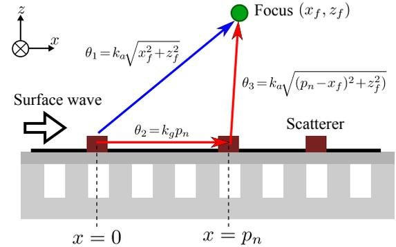
Fig. 3 Focusing principle of our phased array. Surface wave propagates from left to right in this figure along  $x$ -direction. When the phase difference between blue path and red one equals to a multiple of  $2\pi$ , the wave is reinforced and generates a strong focus.
