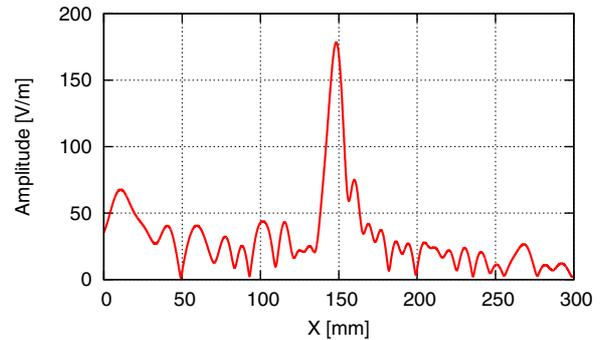
Fig. 6 Magnitude of electric fields  $|E_x|$  along the dotted line in Fig. 4(c).
