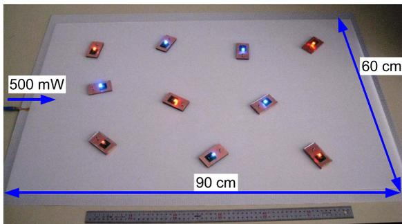
Fig. 1 2DWPT demonstration setup. Ten LED-loaded couplers are distributed on the waveguide sheet.
