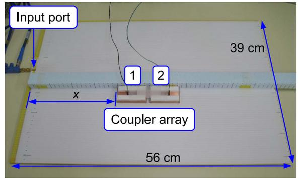
Fig. 5 Position dependence measurement setup. The coupler array consists of two identical couplers. They are aligned in the  $x$ -axis and are mechanically connected with a fixed pitch of 70 mm.
