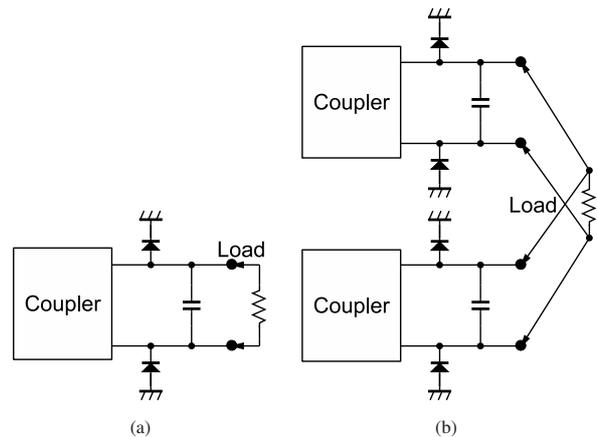
Fig. 6 (a) Single rectifying coupler. (b) Parallel combination of two rectifying couplers. The two outputs are simply combined at the common dc load.
