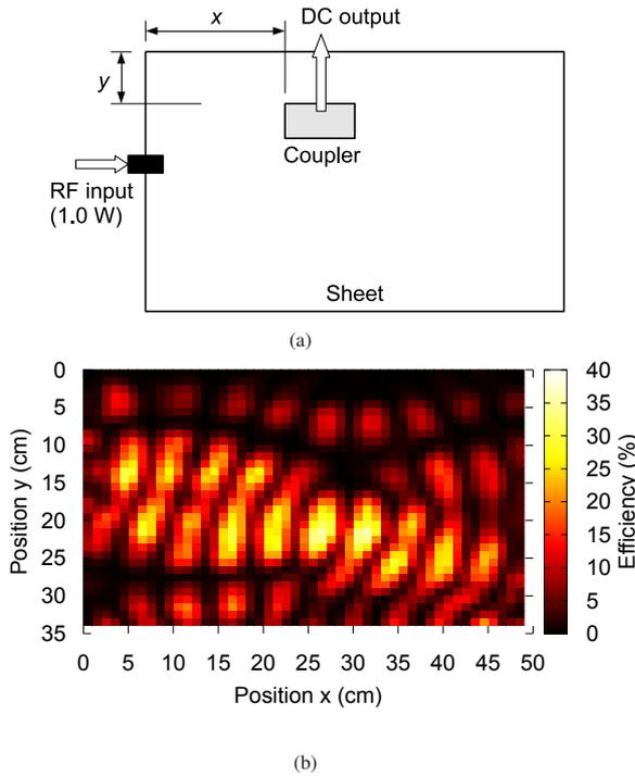
Fig. 2 (a) Position-dependence measurement setup. Dimensions of the sheet and the coupler are  $56 \times 39$  cm<sup>2</sup> and  $64 \times 37$  mm<sup>2</sup>, respectively. (b) Measured RF-to-dc power transmission efficiency with a single coupler. The RF input was 1.0 W at 2.452 GHz.
