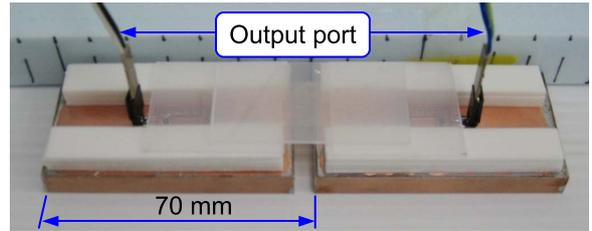
Fig. 4 A complementary coupler pair. Two couplers are mechanically connected with a fixed pitch of 70 mm.
