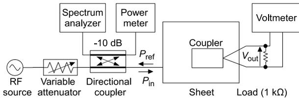
Fig. 3 Measurement setup diagram.  $P_{in}$  was fixed at 1.0 W. The load resistance was fixed at  $1010 \Omega$ , which is an optimum value determined preliminarily.
