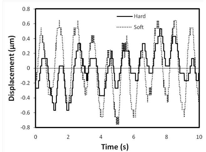
Figure 7. Sinusoidal response of displacement at a center point of two samples.
