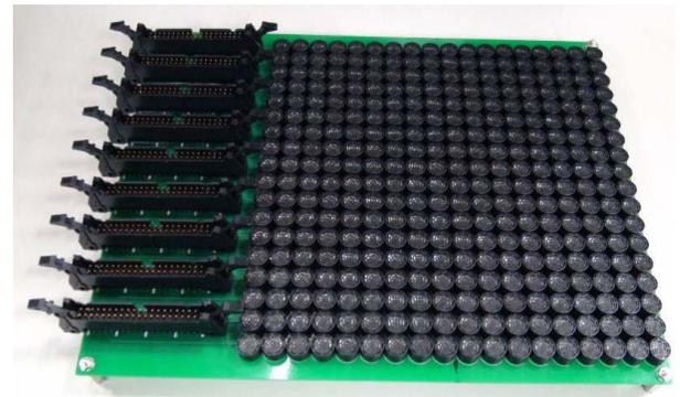
Figure 3. Ultrasound phased array which employed in experiment.
