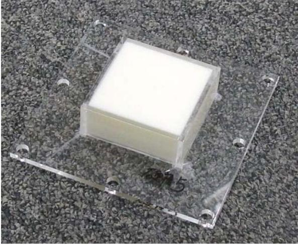
Figure 4. Urethane gel sample of hardness 5 (Asker C) in a container.
