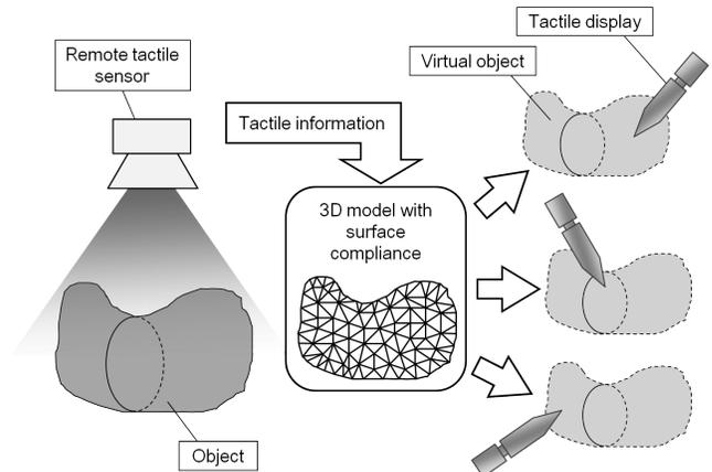
Figure 1. Conceptual image of haptic broadcasting system.
