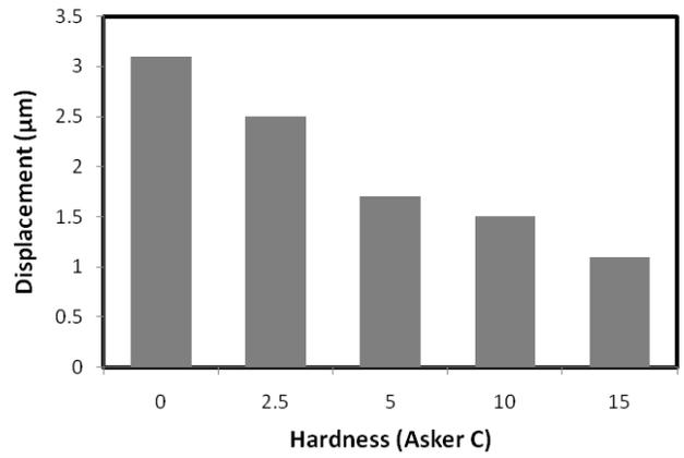
Figure 6. Displacement at a center point of each sample caused by ultrasound acoustic pressure.
