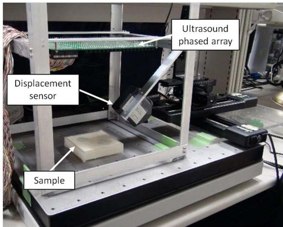
Figure 2. (a) Experimental setup. (b) Picture of experimental setup
