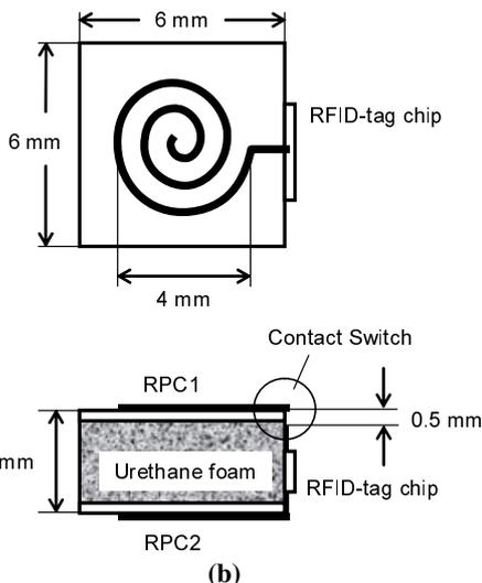
**Fig. 5.** Tactile sensor chip (a) photograph and (b) structure.
