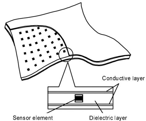
Fig. 1. Sensor skin based on 2DST sheet.
