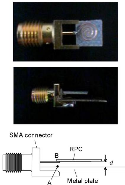
**Fig. 4.** RPC experiment setup. Impedance at the top of the SMA connector was measured with a network analyzer for different distances  $d$ .
