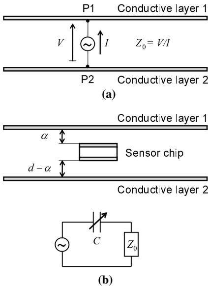
**Fig. 2.** Definition of (a) radiation impedance  $Z_0$  and (b) capacitive connection.
