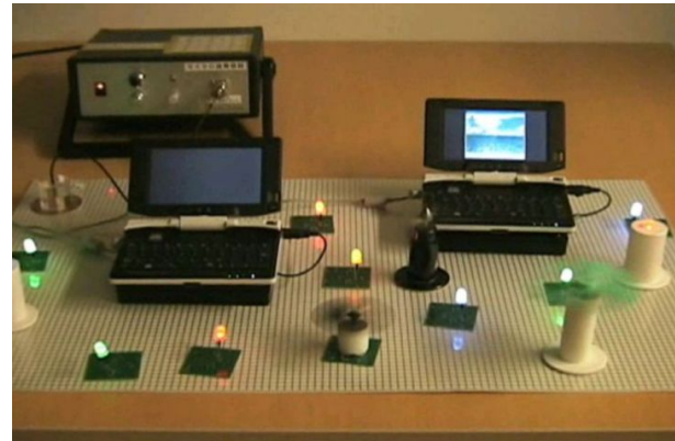
Figure 1: The demonstration of both data transmission and power supply through the Two-Dimensional Communication sheet. The right PC displays the movie data sent by the left one. The LEDs and the small fans receive electricity from the power source shown in the upper-left of the picture via the 2DC sheet.
