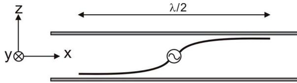
Fig. 4 Two-electrodes-based (I-shaped) model of the new connector
