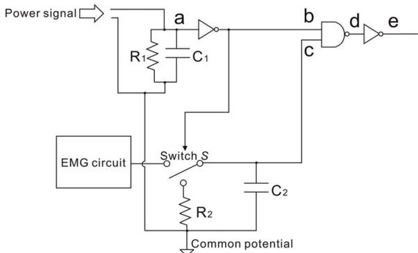
Fig. A-2 Electric circuit that achieves the TDM method with low power consumption.
