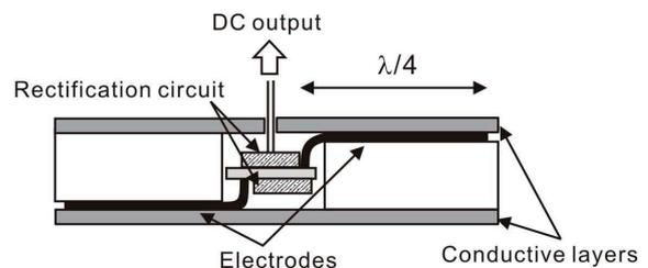
Fig. 3 . Cross section of the new connector.
