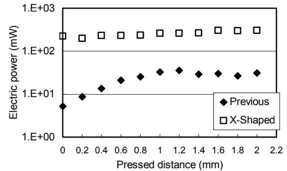
Fig.8 Received electric power depending on the sheet deformation.
