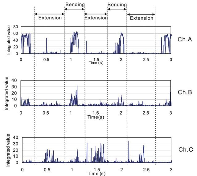
Fig. 11 Demodulated signals. The channel A and B were set upon the muscle related to the bending motion of the wrist. The channel C was set upon the muscle related to the extension of the wrist.
