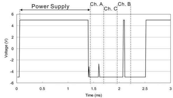
Fig. 10 Observed signal at the power detecting circuit.
