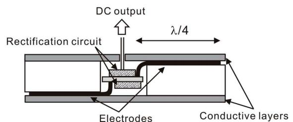
Fig. 3 . Cross section of the new connector.
