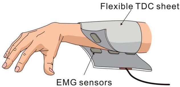
Fig. 1 Schematic diagram of the wristband-shaped electrode array for electromyography
