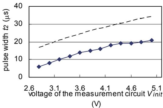
Fig. A-4 The relationship between the voltage of the EMG measurement circuit and the pulse width.
