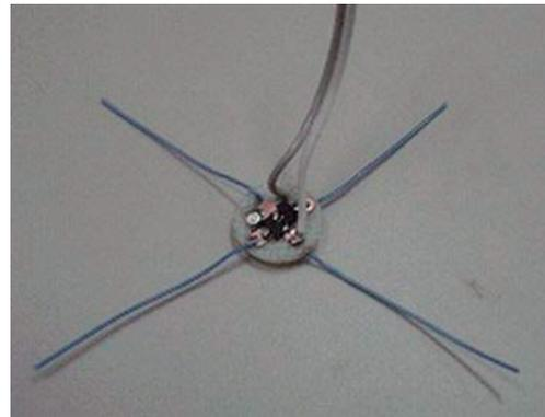
Fig. 2. The new connector having four thin electrodes.
