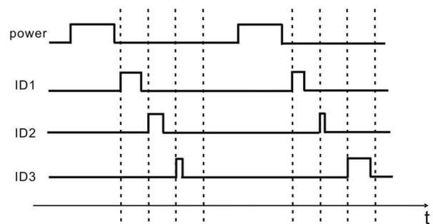
Fig. A-1 Time diagram of the time division multiplexing method. The lateral axis indicates the time. Each sensor has a different delay to the falling edge of the power signal.
