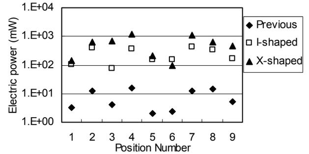
Fig.7 Received electric power with three types of connectors.
