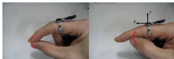
Fig. 2 The difference of the two way of tapping. The axis of the accelerometer is also shown. Left: taps on the distal phalanx (DP tap) Right: taps on the middle phalanx (MP tap).
