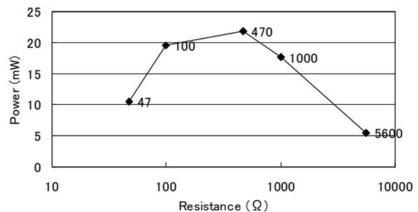
**Fig. 10.** Power consumed at resistance  $R$  for various values of  $R$ .
