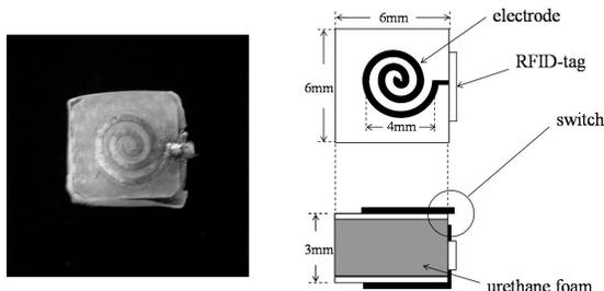
**Fig.11. The photograph (left) and the illustration (right) of the tactile sensor chip.**
