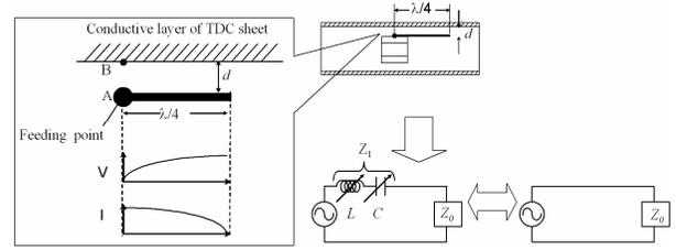
Fig. 3. Schematic explanation of RPC. “ $V$ ” is the vertically measured voltage between A and B, while “ $I$ ” is the horizontal current in the electrode.
