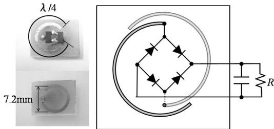
**Fig. 7.** Illustration of power receiving unit. Photograph of the electrode (left) and diagram of the rectification circuit connected to the electrode (right).
