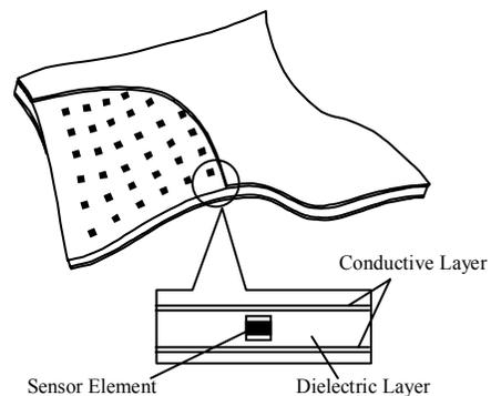
**Fig. 1. Illustration of sensor skin based on Two-Dimensional Signal Transmission (2DST) sheet.**
