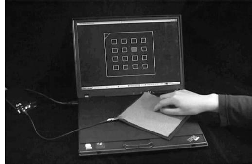
**Fig. 13. The sensor element reacts when the sheet is pressed.**
