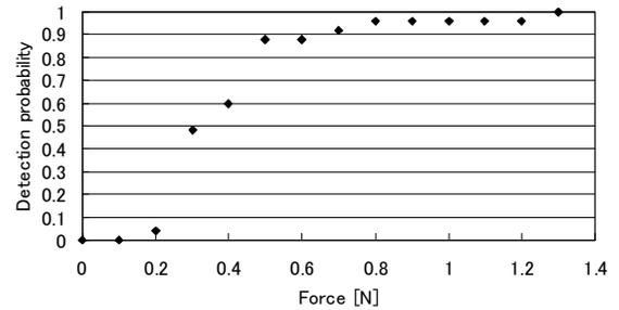
**Fig. 14. Relationship between detection probability of the sensor ID and applied force to the sensor.**
