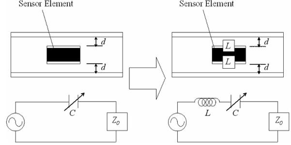
Fig. 2. Illustration of the proximity connection.
