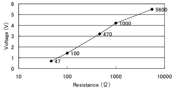
**Fig. 9.** Output voltage at resistance  $R$  for various values of  $R$ .
