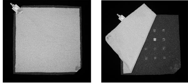
**Fig. 12. The prototype of 2DST sheet (left) and the sensor element put into the sheet (right).**
