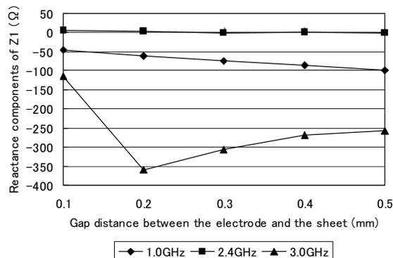
**Fig. 5. Reactance components of  $Z_1$  for various  $d$  of the spiral electrode**
