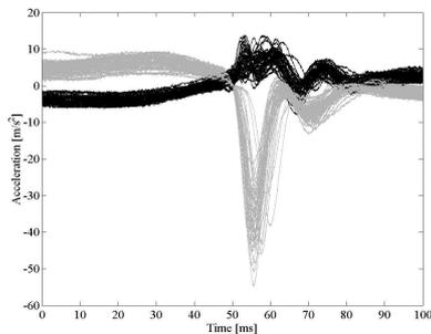
Fig. 4 The observed accelerations for Subject 1 induced by MP tap. The black line is the acceleration of z-axis. The gray line is the acceleration of x-axis. Fifty results are overlaid.
