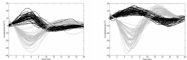
Fig. 7 The observed accelerations for Subject 3 induced by DP tap(Left) and MP tap(Right).
