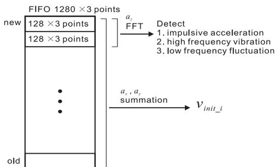
Fig. 11 A diagram of the acceleration data in a FIFO.
