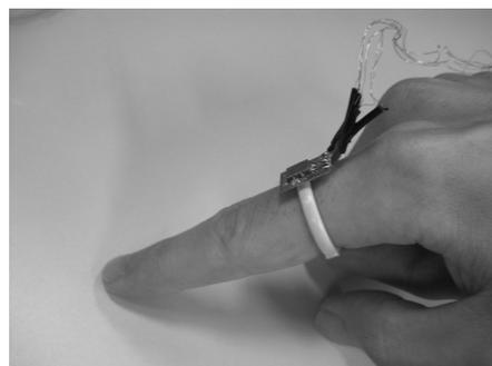
Fig. 1 The finger ring device
