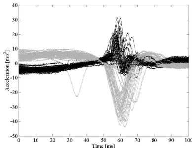
Fig. 3 The observed accelerations for Subject 1 induced by DP tap. The black line is the acceleration of z-axis. The gray line is the acceleration of x-axis. Fifty results are overlaid.
