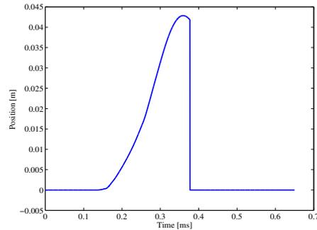
Fig. 12 Calculated position of the finger. The horizontal axis represents time. The vertical axis represents the position. The results were calculated based on the proposed algorithm with the acceleration data shown in Fig. 10.
