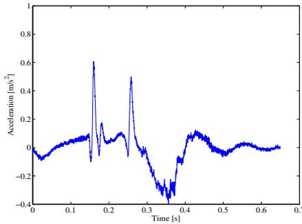
Fig. 10 Observed acceleration during the user is rubbing the finger on a desktop
