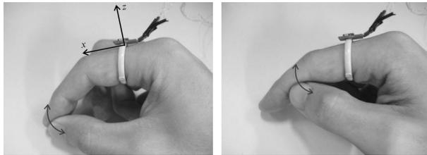
Fig. 2 DP tap (Left) and MP tap (Right). The axes shown in the left figure represents the x- and z-axis of the accelerometer.
