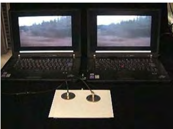
Fig. 16 The left personal computer were played a video transmitting the video signal to the next computer. Signal transmission through the 2DST sheet and a couple of proximity connectors was successful.
