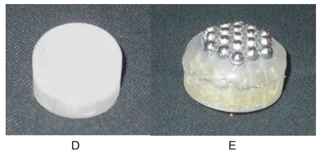
Figure 15: Two reference objects. A smooth surface with the curvature radius of 10 mm (D), and an uneven surface with 19 steel balls with the radius of 2.5 mm (E).
