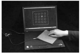
Fig. 13. The sensor element reacts when the sheet is pressed.
