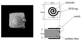
Fig.11. The photograph (left) and the illustration (right) of the tactile sensor chip.
