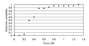
Fig. 14. Relationship between detection probability of the sensor ID and applied force to the sensor.
