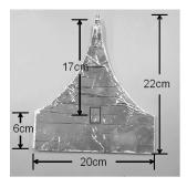
Fig. 6. Photograph of 2DST sheet used in the experiment. The square marked at 17 cm from feeding point indicates the location where a rectification circuit was put.
