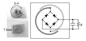
Fig. 7. Illustration of power receiving unit. Photograph of the electrode (left) and diagram of the rectification circuit connected to the electrode (right).
