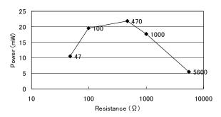
Fig. 10. Power consumed at resistance R for various values of R.
