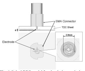
Fig. 4. Spiral RPC model for simulation analysis Table 1. The calculated impedance  $Z_1$  of the spiral electrode for various gaps d
