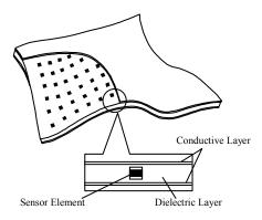
Fig. 1. Illustration of sensor skin based on Two-Dimensional Signal Transmission (2DST) sheet.
