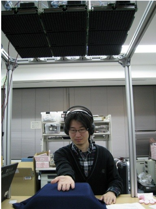
Figure 9: Picture of the identification experiment. On the top of the cabinet was the 9-unit AUTD mounted.
