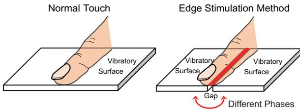
Fig. 1 Schematic of edge stimulation method. Two plain flat surfaces of vibrators in close proximity vibrate in different phases.
