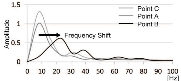
Fig. 8 Spectral analysis on the strain wave of analysis result. Point B has doubled frequency against the vibrator input 10 Hz.
