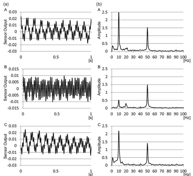
Fig. 5 Experimental results. (a). Skin sensor output at each strain gage position. (b). Spectral amplitude of each signal.
