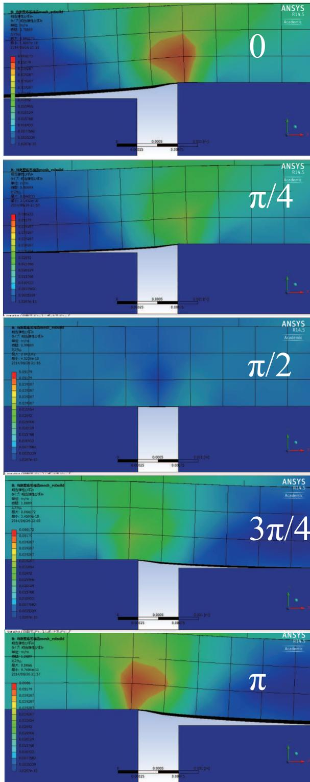
Fig. 9 Animation of dynamic analysis. Full-wave filtering effect is observed between the skin and the vibrators vibrating in opposite phases.
