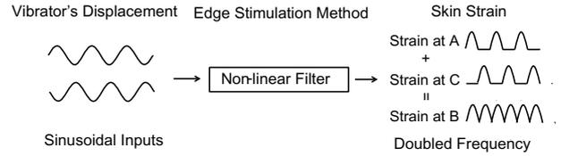
Fig. 10 Schematic of the ES non-linear filter.
