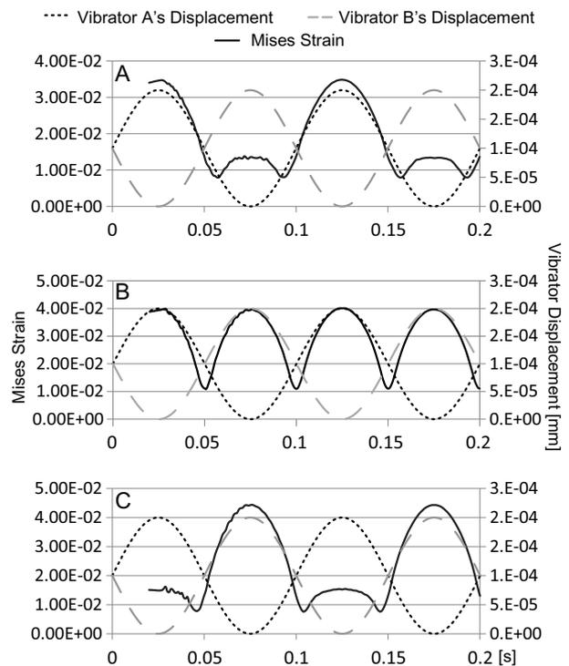
Fig. 7 Dynamic deformation analysis result. Black lines show the strain behavior at each point and dashed/dot lines show the vibrator displacement
