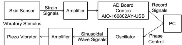
Fig. 4 System of the measurement.
