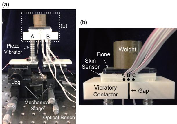
Fig. 3 Skin model sensor. (a). Whole experimental system. (b). Conditions around the skin sensor.
