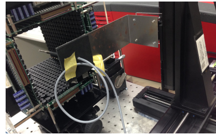
Figure 7: The scene of experiments to measure the actual pressure distribution. The microphone whose diameter is 1/4 inch are mounted on 3-axis motorized stage and was pointed in parallel with phased array.
