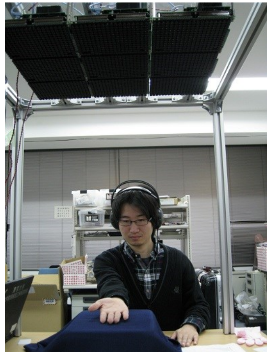
Figure 1: Our newest system of the 9-unit AUTD. The total area of the 3 by 3 units is 57×45cm 2 . Vibrotactile sensation is produced on the user's palm by focused ultrasound emitted from the transducer array mounted above the user.
