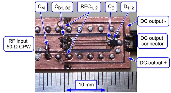
Fig. 5. A fabricated example. The dimensions are smaller than  $20 \times 10 \text{ mm}^2$ .  $\text{RFC}_{1,2}$  are 3-mm diameter, 3-turned coils made of a 0.26-mm thick tinned wire, and are used for the RF isolation and the dc connection.
