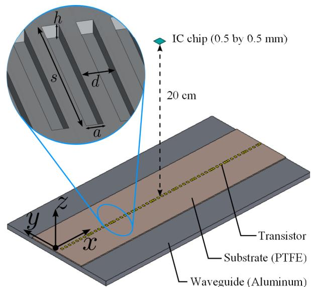
Fig. 1 Schematic view of our phased array. A sub figure in the upper left circle shows the waveguide structure under the PTFE substrate. In this research we transmit 1mW to the IC chip at a 20 cm distance from the phased array.
