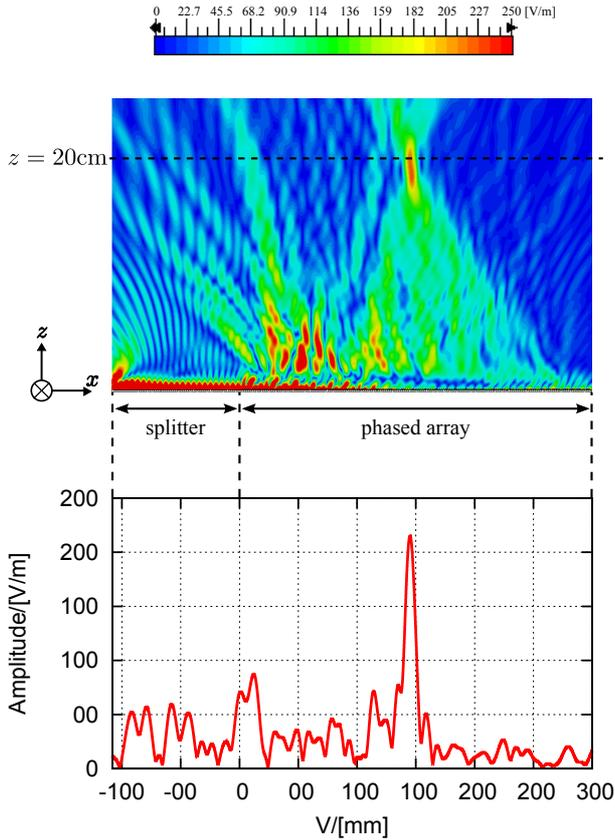
Fig. 9 (Top) Simulated electric field amplitude  $|E_x|$  distribution map for the 30-GHz two-dimensional phased array with splitter. (Bottom) Magnitude of electric fields  $|E_x|$  along the dotted line in upper figure.
