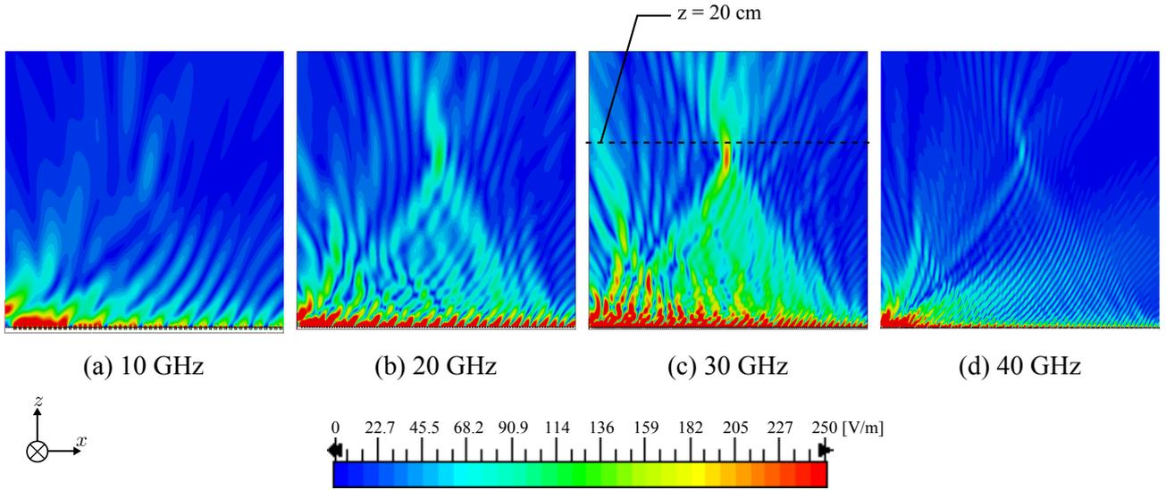
Fig. 4 Simulated electric field amplitude  $|E_x|$  distribution map for four cases. As frequency becomes high, a focus is generated finely. This is because the number of scatterer increases as frequency is high. Thus in terms of the performance of phased array, we need to use electromagnetic wave with high frequency.
