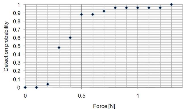
Fig. 9. Sensor ID detection probability vs. force applied to sensor.
